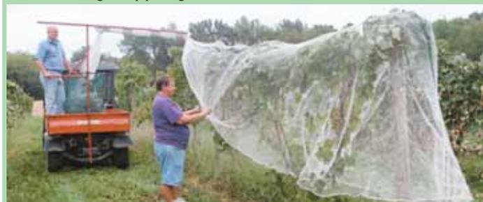
T-shaped metal support frame bolts on back of utility vehicle. Netting slides out through 8-in. dia. pvc pipe at top of frame.
