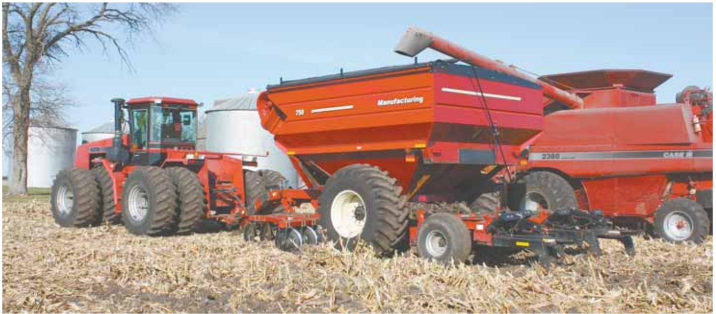
John Standley and his father Calvin built this one-of-a-kind "tillage cart" by adapting the disk and shank components from a 15-ft. chisel plow onto the reconstructed frame of a 750-bu. grain cart.
