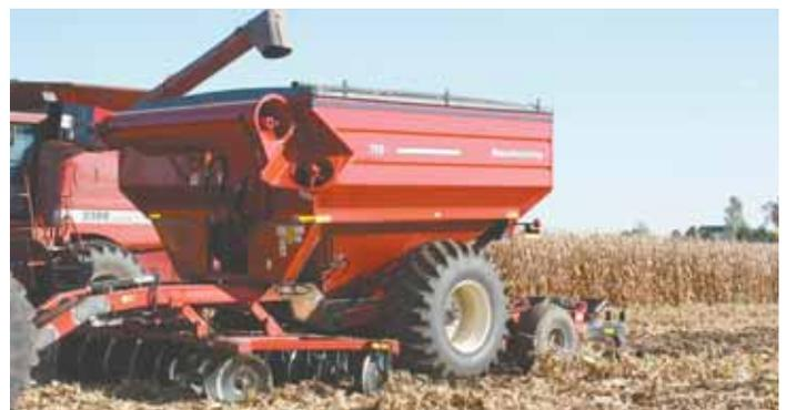
Rig collects grain from a combine and does tillage in a single pass to save trips across the field, minimizing the time it takes to complete fall field work.
