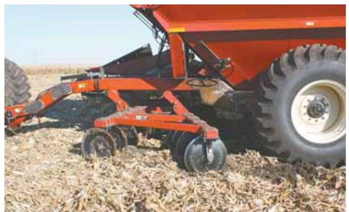
Two disk gangs from the chisel plow mount under cart's bridge frame at an 18-degree cutting angle. Gangs mount on hinges that allow 16 in. of up and down travel.
